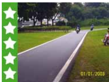
Fully separated facility with one way flows, no side friction, good delineation and forgiving roadsides, 80 km/h
